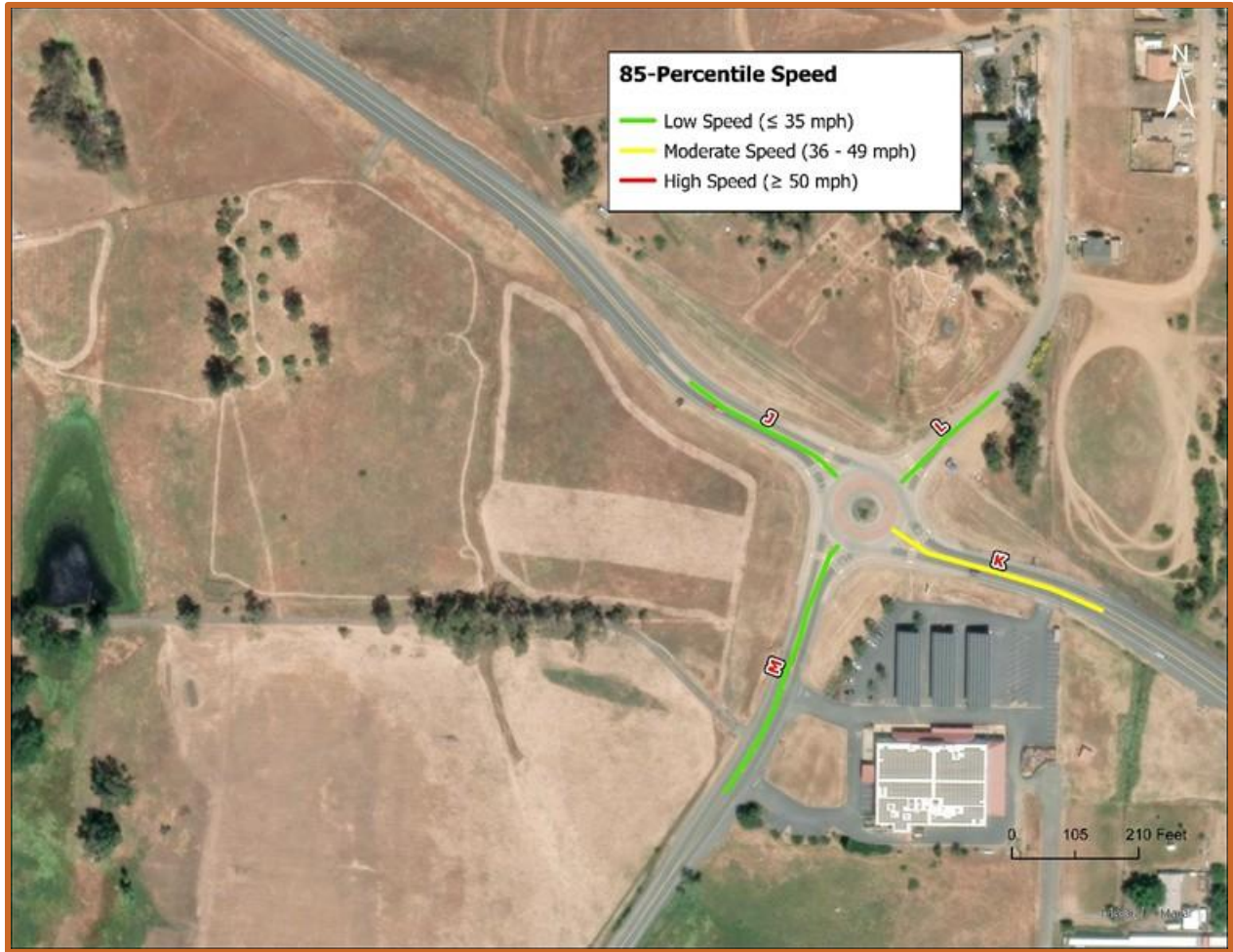
Figure 20. Daily Speed Survey Results Near SR-20/Pyle Road Roundabout
