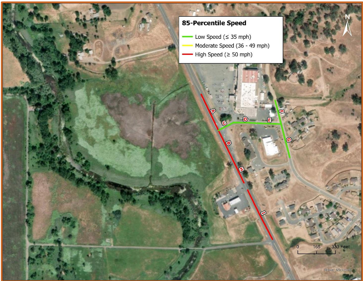
Figure 19. Daily Speed Survey Results Near Robinson Rancheria
